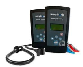
The device consists of a transmitter (IC2G-TX) and a receiver (IC2G-RX), and it is easy to use: the transmitter (TX) is connected to an LVdistribution cable and the receiver (RX) is used to identify or locate that cable upstream, towards the MV/LV transformer.
